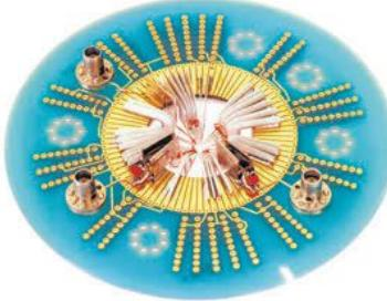
Through unique modular design techniques, hundreds of low frequency probe needles and a variety of microwave probes with operating frequencies from DC to 40, 67, or even 110 GHz can be custom configured to your layout.
