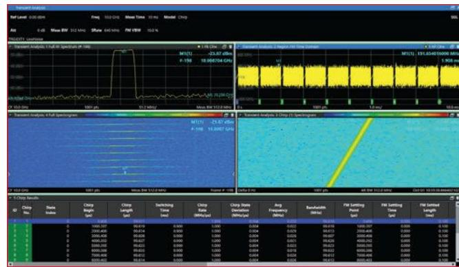
▲ Fig. 2 Example of pulse modulation analysis with K710 transient analysis.
