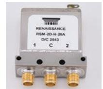
Conquer the harshest environments with DC to 18 GHz RF switches from Renaissance Electronics, an AEM company. Delivering exceptional performance for ground, sea, airborne and space applications, these switches are hermetically sealed for maximum protection and unwavering signal integrity. Available in Failsafe and Latching configurations, and adaptable from SP2T through SP8T configurations to meet your precise needs.
