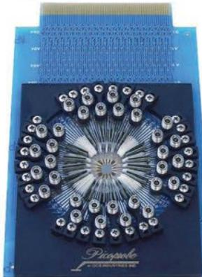
Our patented probe structures provide the precision and ruggedness you require for both production and characterization testing. And only Picoprobe® offers the lowest loss, best match, low inductance power supplies, and current sources on a single probe card.
