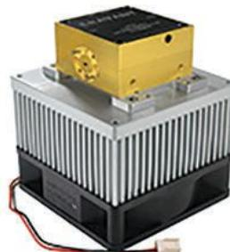
Providing 18 dB small-signal gain across the 75 to 110 GHz range, model SBP-7531141833-1010-C1-HR delivers +33 dBm saturated output power. The amplifier operates from a single +18 VDC supply and features WR-10 waveguide ports with anti-cocking flanges for reliable alignment.
