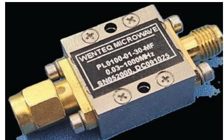
Model PL0100-01-30 is a PIN-diode based power limiter module designed to protect RF systems from ESD and input power surge damages up to 30 dBm power. It operates in the frequency range from 30 kHz to 1.0 GHz with 0.2 dB typical insertion loss and 1.2:1 max. VSWR. Compression starts when the input power reaches +7dBm and the leaked power at +27 dBm is less than +13 dBm. The package size of the amplifier is 0.75 x 0.70 x 0.4 in.
