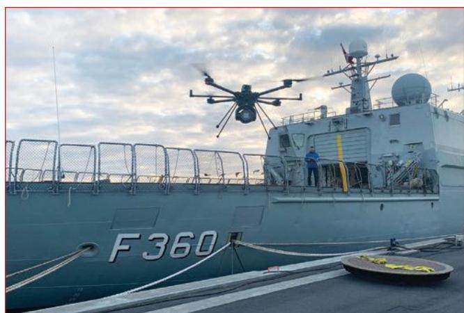
▲ Fig. 1 A UAV with an RF payload flying near a ship.
